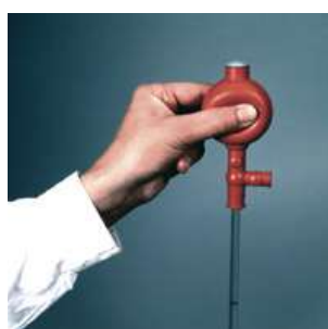
1. Evacuate the air by pressing the bulb, as the drawing indicates.
