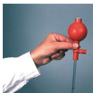
2. Intake by pressing on point B ↻
