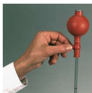
3. Drain the liquid by pressing on point A ⬇
